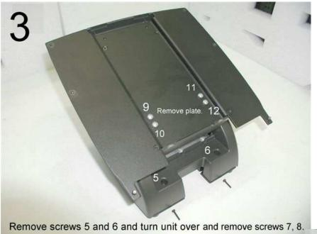
•Referring to picture 3, remove screws 5 and 6 and turn unit over.
